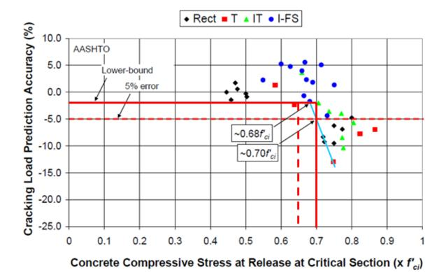
According to descriptions of relevant research provided in Birrcher, et. al. [2], the  $0.65f'_{ci}$  recommendation was based on tests of specimens that were either uniformly loaded in compression or did not have lateral bending concerns as noted above. Therefore, the experimentation represents a "global" stress condition in the specimens. Bending about the minor axis does not result in a net change in these "global" stresses, but introduces peak stresses at the extremities of the member.
