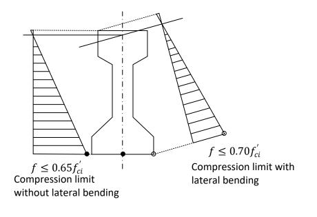
Figure 5.2.1-1 – Application of compressive stress limits for lifting and shipping.
