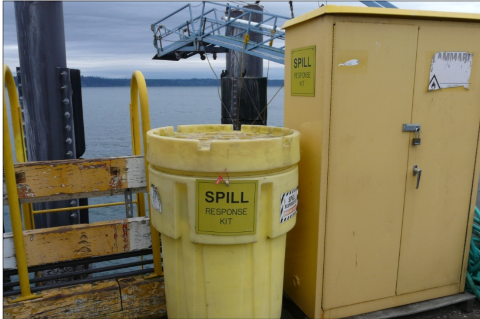
Vashon Ferry Terminal Oil Spill Response Kit Exhibit 440-13
