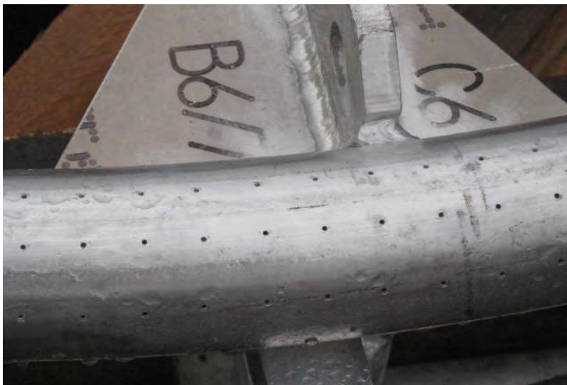
Figure 7: Photo of bubble curtain ring system used for this project and the bubble curtain hole spacing pattern
