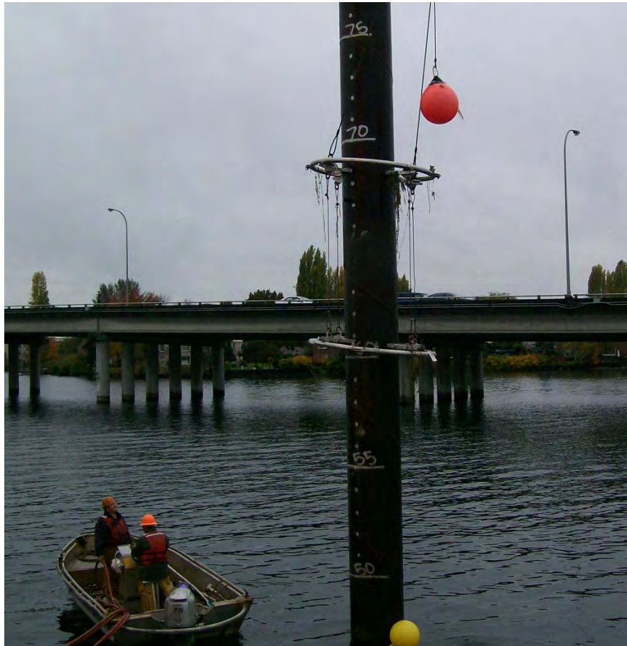
Figure 8: Photograph of the bubble curtain being deployed
