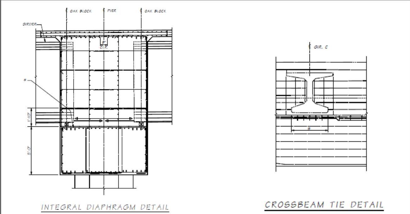
Figure 3: Lower Crossbeam Ties
