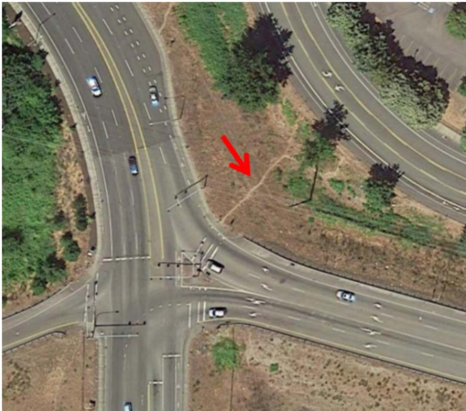
Figure 3-2: Desire line trails. User-made trails reduce the distance pedestrians must take between destinations. This path connects to a large freeway interchange in Olympia, WA. Both sides of the interchange offer housing, services, and employment centers. Trails such as this may be very useful to those with the ability to follow them, but they are neither approved routes nor accessible to all users.
