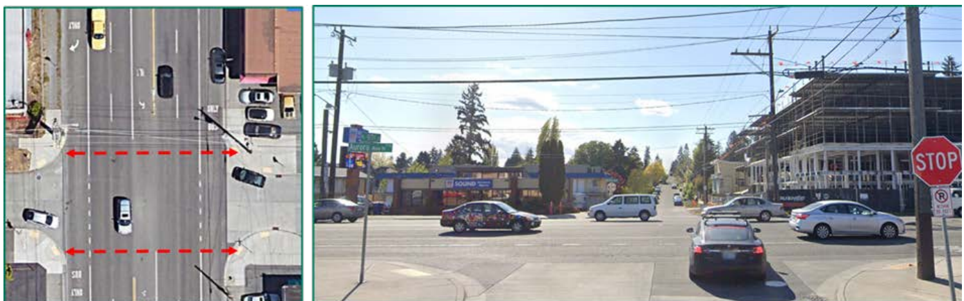
Figure 3-8: Pedestrian level of traffic stress. Like Bicycle LTS, PLTS can apply to trips along and across motor vehicle lanes. These photos illustrate an example of a PLTS 4 situation on Aurora Avenue in Seattle. Crossing is legal here, which the curb ramps highlight, but with a posted speed of 40 mph, high traffic volumes, four travel lanes, and three special purpose lanes, it would be a challenging crossing for any adult. Marked crossings with pedestrian signal phases are available two blocks north or one block south of this location, but these options add to a pedestrian’s trip distance, which could be a factor for some people.
