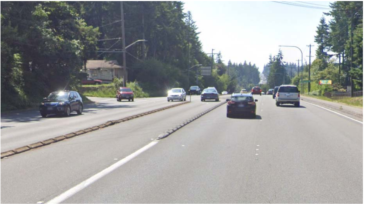
Figure 3-14: Segment gaps. Segment gaps were found throughout the state, with some of the most challenging for bicyclists found in larger cities. State Route 104 has multiple lanes, high traffic volumes, and relatively high-speed traffic. The roadway lacks dedicated space for people on bikes; the best solution may or may not be on the state highway in locations like this. This segment has a sidewalk on one side, so it could still pose a challenge for some pedestrians depending on which side of the road they are on at the beginning or end of their journey. Image source: Google Maps.
